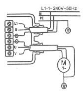
Wiring diagram for connection of single phase 240V pumps up to 1.5kW.
